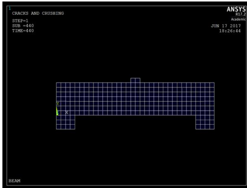
Figure 5-24 Concrete Crack Plot at 2933 lbs. Before First Crack
