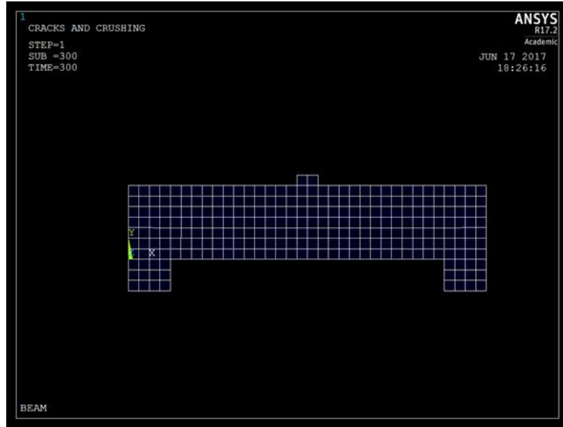
Figure 5-23 Concrete Crack Plot at 2000 lbs. in Linear-Elastic Range
