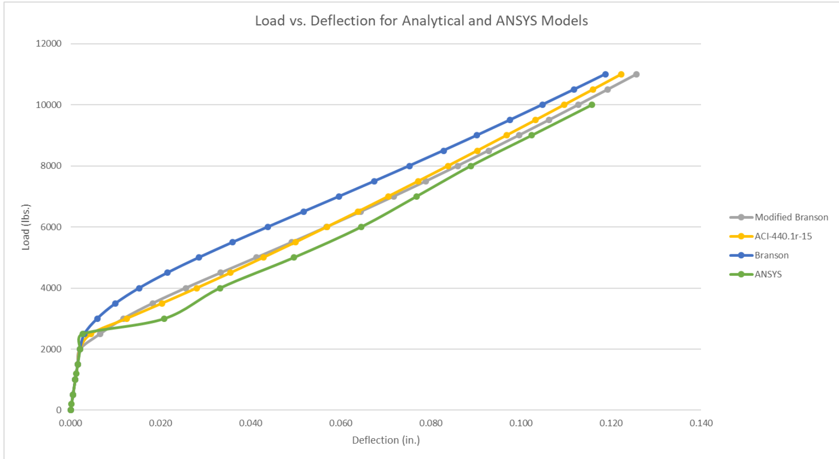
Figure 6-2 Load vs. Deflection for Analytical and ANSYS Models
