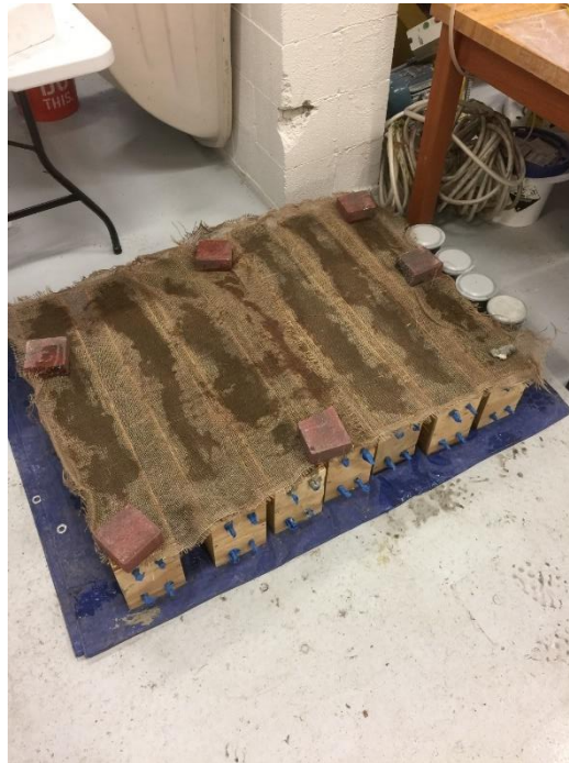
Figure 3-5 Curing of Concrete Beams with a Burlap Cover
