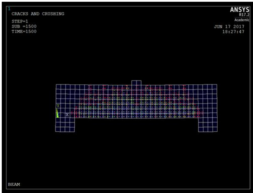
Figure 5-26 Concrete Crack Plot at 7500 lbs. in Nonlinear Range
