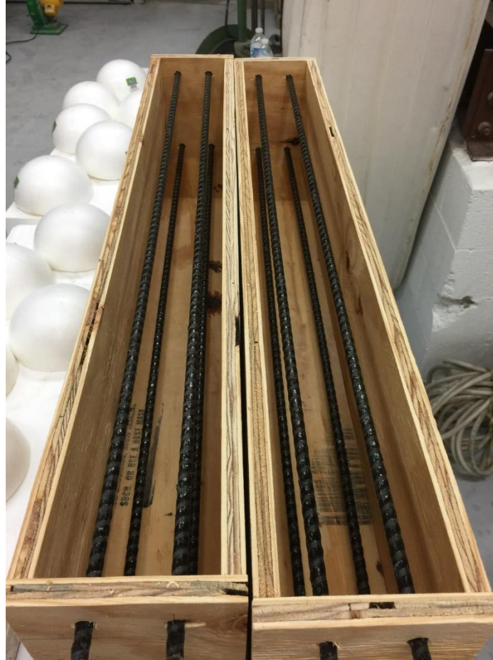
Figure 3-3 BFRP Reinforcements Positioned in Plywood Forms
