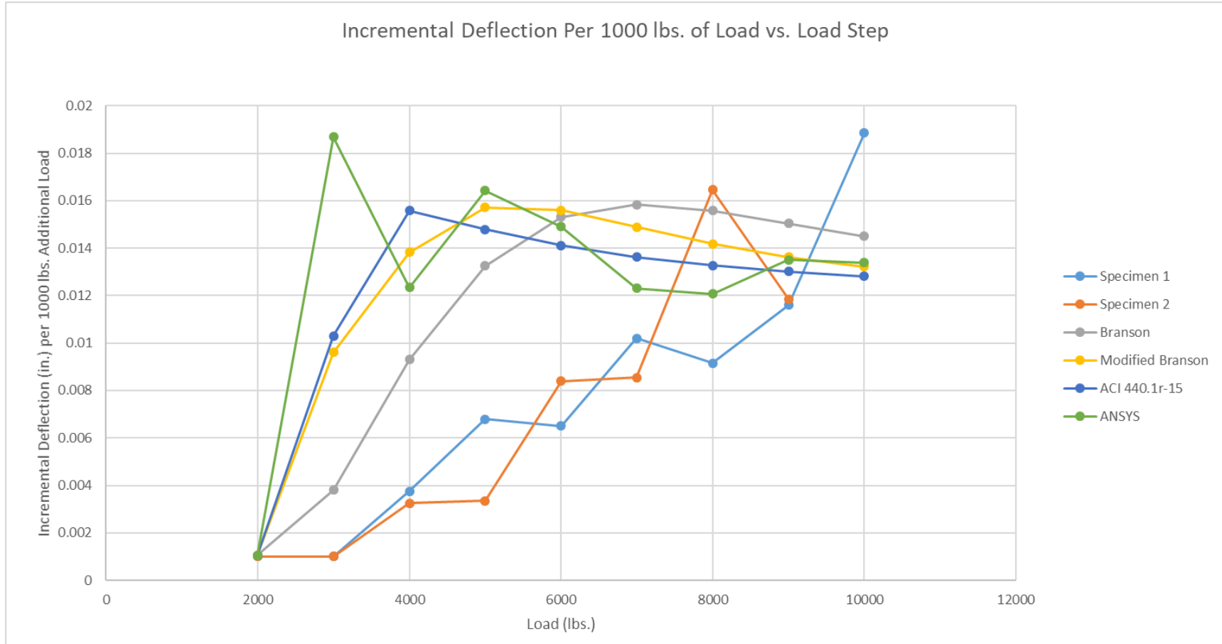
Figure 6-5 Incremental Deflection for 1000 lbs. Incremental at Each Load Step
